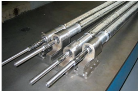
A set of four cartridges for the Q1 and Q3 repair, each consisting of an Invar rod inside an aluminum tube.
