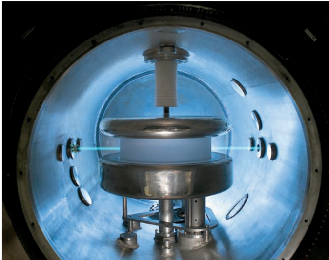
The storage bottle inside the four-fold mu-metal shielding of the instrument used in the high-precision measurement of the neutron's electric dipole moment at ILL. (ILL/Artechnique.)
