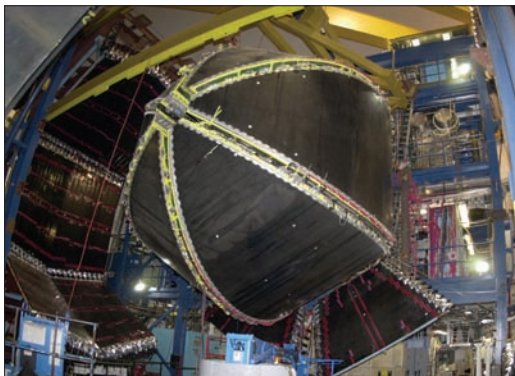
Fig. 1. The CLAS spectrometer, shown with the outer detector arrays moved away from the inner tracking detectors. (Courtesy Jefferson Lab.)
